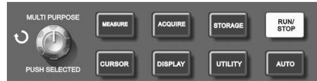
Figure 2-27 Function key for the sampling system (auto measurement)
