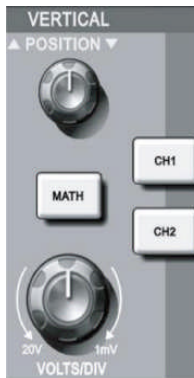
Figure 1-9 Vertical control zone on the front panel
