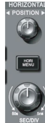
Figure 1-10 Horizontal control zone on the front panel
