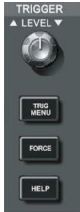
Figure 1-11 Trigger menu control zone on the front panel
