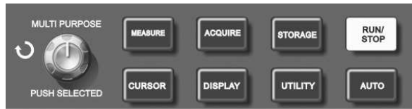
Figure 2-17 Function key for the sampling system
